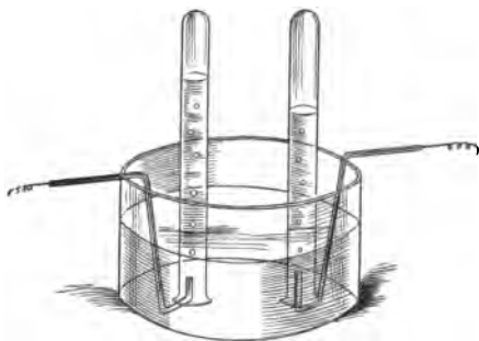
FIG. 212. — The decomposition of water.
